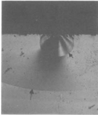
Figure 1 Fracture mirror after failure in a lifetime test. Inner contour: initial crack size after indentation test. Outer contour: crack size at failure.
